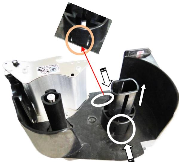
**Method of bushing remove:** use your fingers to press inward according to the arrow direction and take the bushing upward.
