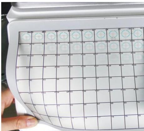
→ Push up the hotkey pad from bottom according to the arrow head.
