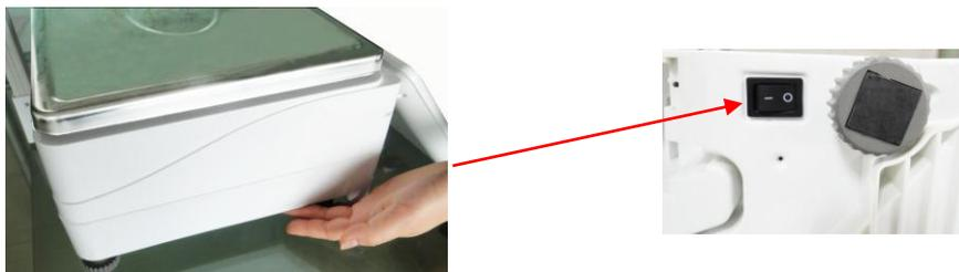
**Press On/Off key at the left bottom of the machine after connecting the electricity**
